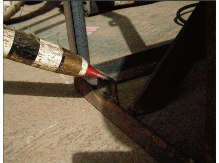
Weld the bike frame in place, lining up the sprockets so the chain will run straight. You will need to bend the drive-side chain stay in order to clear the chain.
