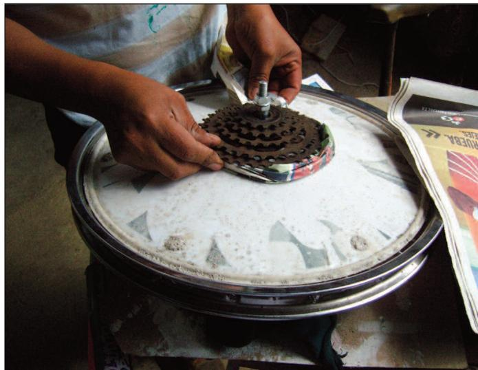
The mould for the concrete is made using a child's bike wheel cover. These are hard to come by, so you may need to improvise. It's kept in place with a cassette and packed with newspaper to prevent leakage.
