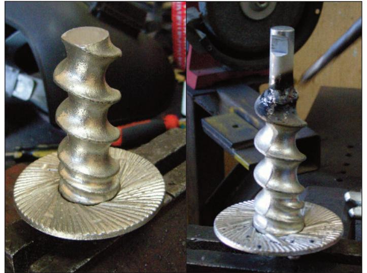
...and part of a "cotted"\* crank axle is welded on in it's place. It must be square. We use electrodes designed for cast steel to weld this part.
