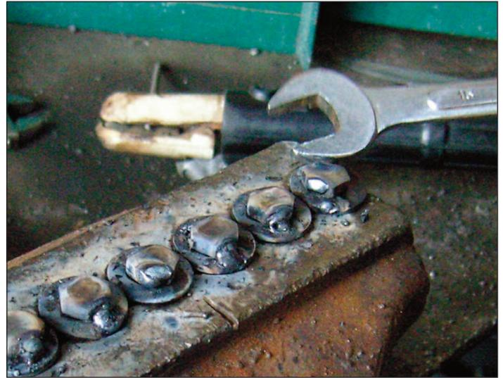
In order to bolt on the handle bars, we weld 8mm bolts onto 20mm washers.
