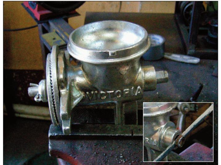
Our adapted axle needs a pipe shim. Insert one if required and trim any excess.
