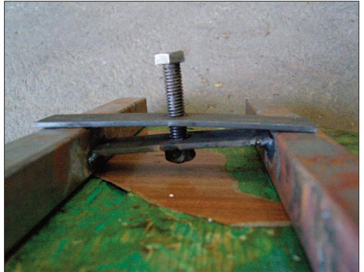
In order to make the seat position adjustable, there is a simple bracket. The nut is welded in place for easy tightening.
