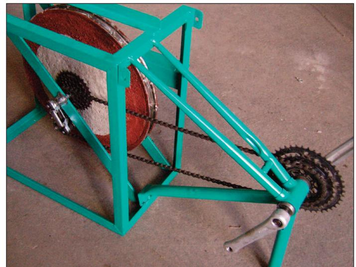
The drive side derailleur is bolted in place as it would be on the bike. However it will need to be filed to fit flush with the frame. We use the old style of derailleur that bolts onto the axel rather than the bike frame.
