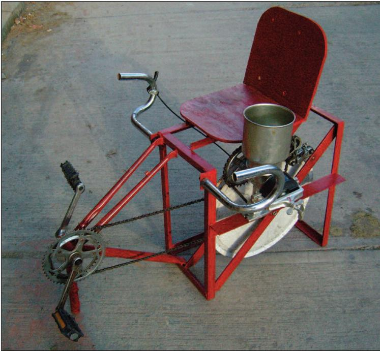
Maya Pedal's best selling "Bicimaquina". This design provides a stable, sit-on pedal power system to drive numerous types of appliance. In Guatemala it's used primarily to thresh and grind corn utilising two locally available, hand powered appliances. Each appliance must first be adapted to pedal power by modifying the drive shaft to incorporate the end of a cottered bottom bracket axel.
