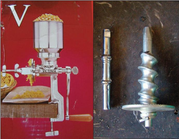
The mill itself is hand operated and table mounted. Remove the central spindle. One end accepts the handle, the other end forms part of the grinding mechanism. The handle part is cut off completely...
