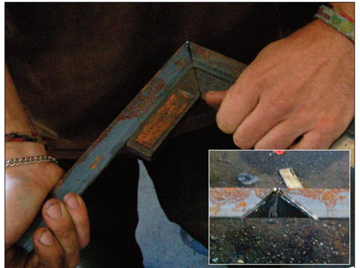
Form the 90 degree corners as shown, cutting, folding and welding the angle iron.
