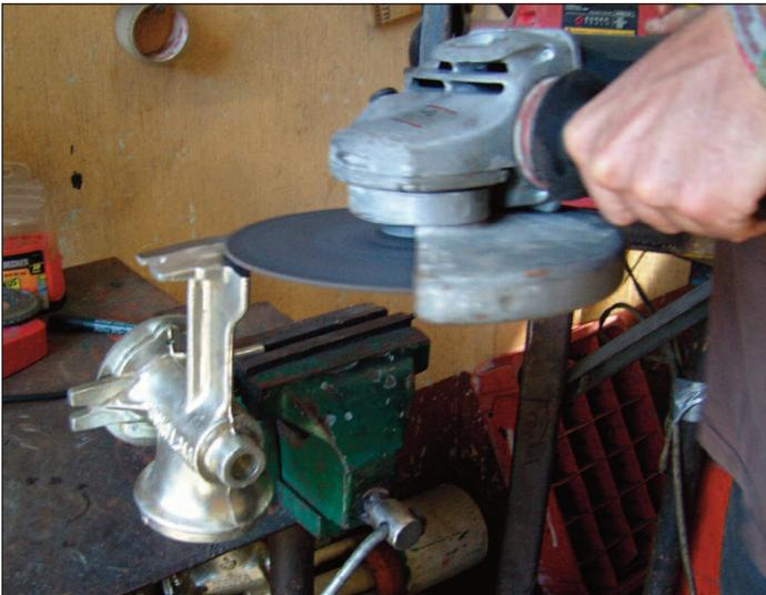
The mill will eventually bolt onto the frame. Remove the table mount as shown, leaving a square, flat edge.
