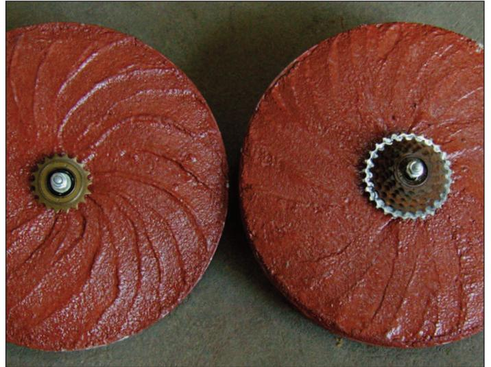
The concrete is painted to protect from moisture. One side accepts a multi speed cassette, the other a single speed sprocket. The axel position will need to be adjusted accordingly.
